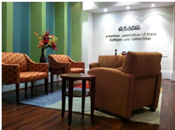
New recycled green vinyl wood flooring alternative was installed for softness underfoot, quiet acoustical control, rolling carts, ease of maintenance and no VOC installation with a click in place plank design.
